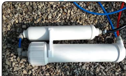
Reverse Osmosis system
